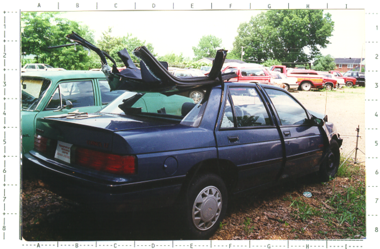
# 45 -- Right back view of 1991 Chevrolet Corsica's undamaged back and right side, except for peeled-back roof and induced FR damage
